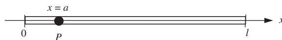
Figure A.4 Point force (point source) acting in the interior of the element.
