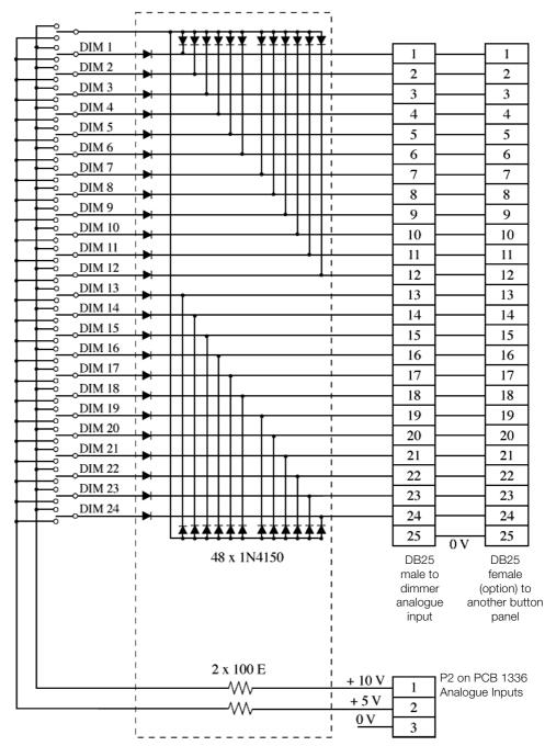
For EURORACK with 18 or 24 dimmers, the + 5 V and + 10 V required for the pushbuttons is supplied from connector P2 on the "Analogue Input Board".
