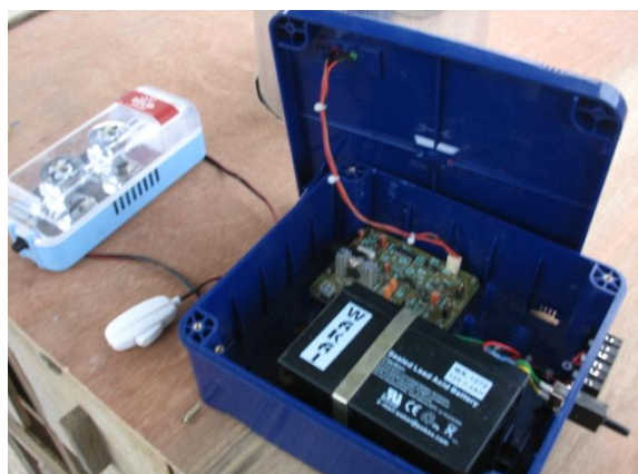
Figure 1: Small SHS (WLED lamp, switch, battery and charge controller circuit)
