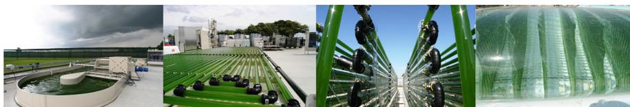
Figure 3. The four main reactor types, at AlgaePARC Wageningen UR. From left to right: raceway pond, horizontal tubes, vertically stacked horizontal tubes and flat panels. With permission of Wageningen UR.
