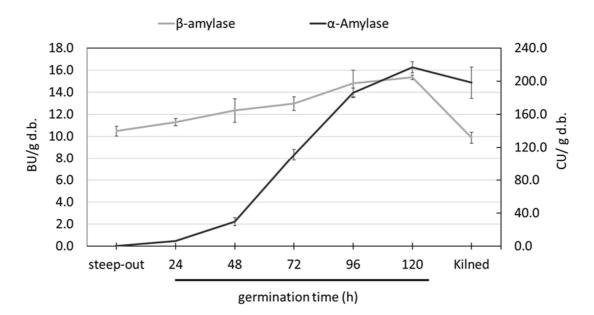
Figure 2.3:  $\alpha$ - and  $\beta$ -amylase activity monitored during germination in the malting barley variety Flagon with rootlets;  $\beta$ -amylase (Betamyl-3<sup>®</sup>Units; BU) is displayed on primary axis whereas  $\alpha$ -amylase (Ceralpha-Units; CU) is displayed on the secondary axis. Data are the mean ±SD of 3 biological and 2 technical replicate measurements.
