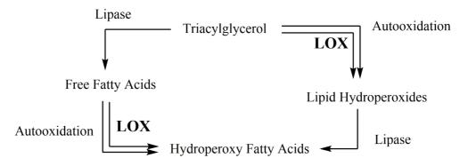
Figure 1.5: The formation of hydroperoxyl fatty acids through enzymatic lipidoxidation (lipase, lipoxygenase (LOX), and autooxidation (Baert et al., 2012, Kobayashi et al., 1994).
