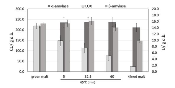
Figure 2.5: Model data showing the impacts of heating green malt at 65 °C for periods of up to 1 h. The primary axis displays  $\alpha$ -amylase activity (Ceralpha units/ g d.b).; the secondary axis displays  $\beta$ -amylase (Betamyl-3<sup>®</sup> Unit/ g d.b.) and lipoxygenase activity (U/g d.b).; Data are predicted responses given by the model fitted to experimental results.
