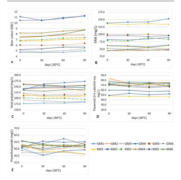
Figure 5.3: Evolution of A) beer colour, B) free amino nitrogen, C) total polyphenols, D) flavanoid and E) proanthocyanidin concentration during ageing of beer (30°C). Results are the mean of 3 technical replicate measurements.
