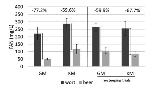
Figure 3.6: FAN levels (mg/L) in worts and beers prepared from green malt, re-steeped green malt and their corresponding reference malt. The average percentage uptake (%) from pitching wort to matured bottled beer is indicated. Data are the mean SD of 3 biological with each 3 technical replicate measurements; GM = green malt, KM = kilned malt.
