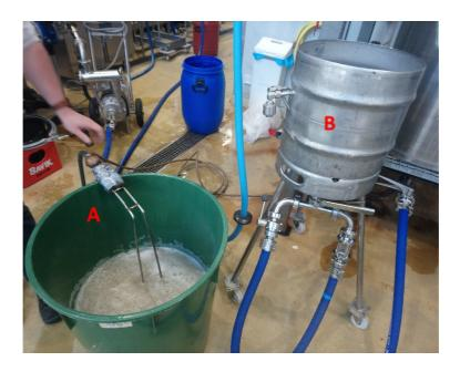
Figure 3.5: Heating of re-steeping water using an immersion heater (A); water tank connected to mash kettle (B)
