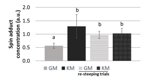
Figure 4.8: Formation of spin adducts in beers measured by ESR. Beer samples were forced aged for 90 min at 60°C (T90 values) after the addition of PBN (30 mM final concentration). Values corrected for TEMPO used (10 μm) and presented as mean ±SD of 3 biological replicates with each 2 replicate measurements. Statistics: One-Way ANOVA with Tukey's post-hoc test. a-b superscripts represent the ANOVA post-hoc groupings.
