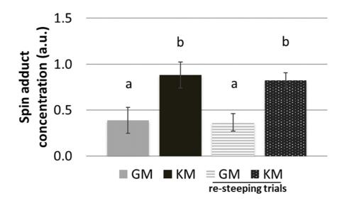
Figure 4.7: Formation of spin adducts in pitching wort samples measured by ESR. Wort samples were forced aged for 120 min at 60°C (T120 values) after the addition of PBN (30 mM final concentration). Data corrected against a TEMPO standard (10  $\mu$ M) and presented as mean ±SD of 3 biological replicates with each 2 replicate measurements. Statistics: One-Way ANOVA with Tukey's post-hoc test. a-b superscripts represent the ANOVA post-hoc groupings.
