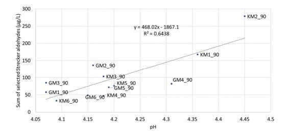
Figure 5.12: Concentrations of the sum of selected Strecker aldehydes (2-Methylpropanal, 2-methylbutanal, 3-methylbutanal, methional and phenylacetaldehyde) measured in aged beers (30°C, 90 days), plotted as a function of the corresponding pH in the beers.
