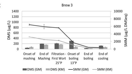
Figure 3.3: DMS and S-methyl methionine (expressed as DMS equivalents, μg/L) monitored in three individual brewing processes using green malt and the corresponding reference (pale) kilned malt. Data are the mean ±SD of 2 technical replicates.
