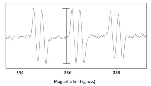
Figure 1.10: ESR spectrum of a PBN spin adduct. The amplitude of the third peak is recorded.
