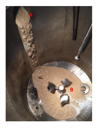
Figure 3.2: Mash kettle; Inlet and thick (1:2.2) green malt 'mash' (A), homogeniser at the bottom of the mash kettle (B)
