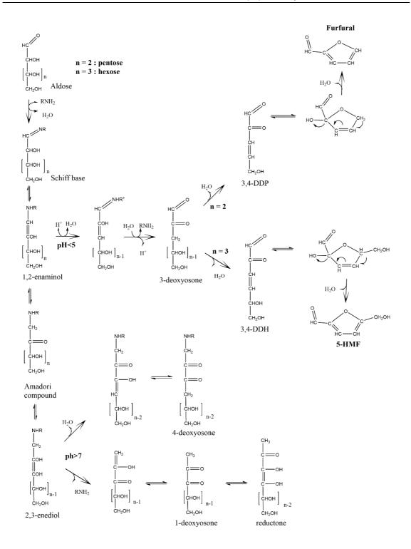
Figure 1.7: Overview of the Maillard reactions yielding 5-hydroxymethylfurfural (5-HMF) and furfural according to Baert et al. (Baert et al., 2012); 3,4-DDP, 3,4dideoxypentosulose-3-ene; 3,4-DDH, 3,4-dideoxyhexosulose-3-ene; 5-HMF = 5hydroxymethylfurfural
