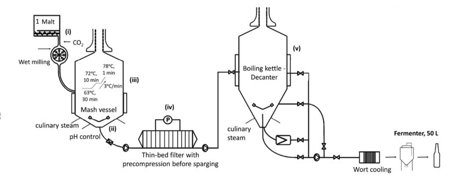
Figure 3.1: Process outline of the KU Leuven brewery; Points i-v indicate critical points when brewing with green malt. i) wet milling; ii) mash agitation; iii) mash conversion vessel; iv) membrane mash filter; v) kettle-decanter.
