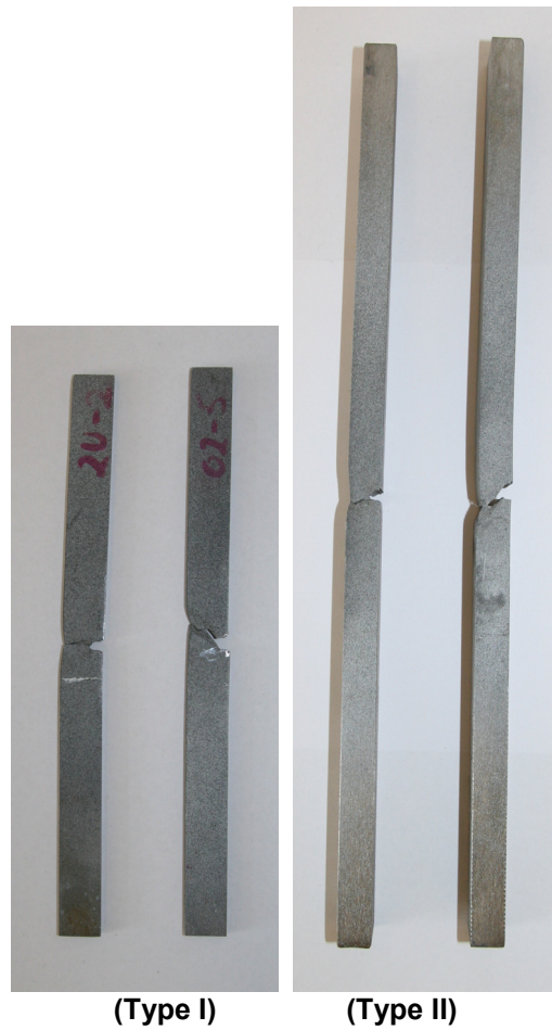
Figure 6. Examples of specimens after tension testing, specimen type I (3 mm width) and specimen type II (24 mm width).
