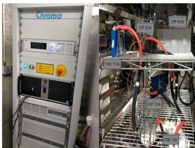
Figure 1. Experimental setup and tested batteries inside the climate chamber
