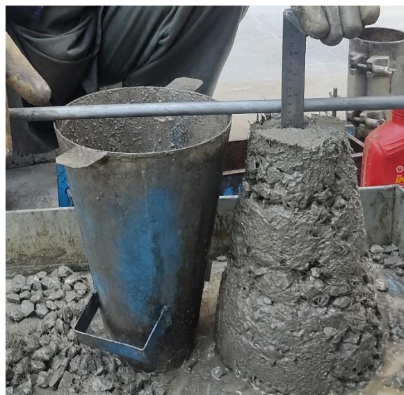
Figure 1. Measuring the value of slump of PUB.
