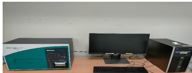
Figure 2. Heat Flow Meter test bench
