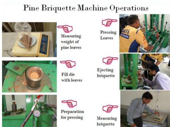
Figure 6 Briquetting on manually operated machine
