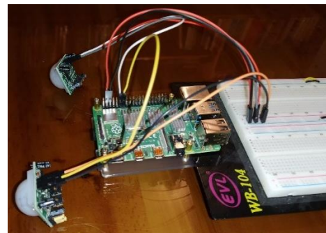
Figure 3. PIR sensors connected to Raspberry Pi 4. Source: Author.
