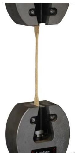
Figure 3. Experimental set-up of tensile test
