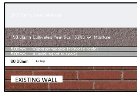
Figure 3: Green Wall Cross Section
