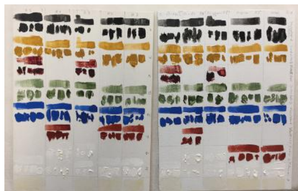
Figure 2 Mock-ups of paints based on different binders made during the workshop. (Photo © Renate Poggendorf.)
