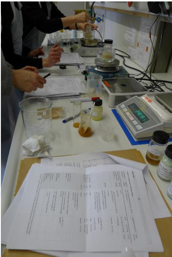
Figure 1 Preparing the Syntonos binding media according to the historical recipe. (Photo © TU München, Lehrstuhl für Restaurierung.)
