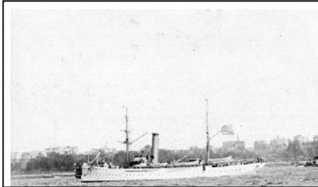
Revenue Cutter Manning 1898-1930. the era of transition from sail to steam. Designed as a cruising cutter for the U.S.R.C.S, built by Atlantic Works of E. Boston, Mass.; commissioned at Boston, 8 January 1898, decommissioned at Norfolk, Va., 22 May 1930; sold to Charles L. Jording of Baltimore, Md. Dec 1930 Displacement, 1,155 tons; Length. 205'; Beam. 32' Drafts, 13'9"; Speed, 15 knots, Armament 2-3" guns & 2 six pounder rapid fire guns.
