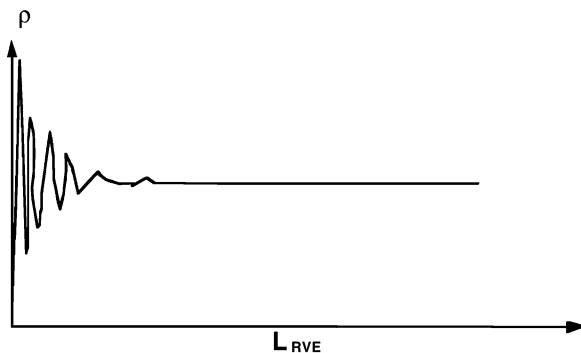
Fig. 7.2 A plot of the values of the macro density as a function of the size L_{\text{RVE}} of the RVE. Note that as the size of the volume V_{\text{RVE}} = (L_{\text{RVE}})^3 is decreased, the value of the density begins to oscillate because the amount of dense solid material in the volume V_{\text{RVE}} is greatly influenced by the occurrence of small voids. On the other hand, as the size of the volume V_{\text{RVE}} = (L_{\text{RVE}})^3 is increased, the value of the density tends to a constant, stable value. The concept for this plot is taken from Prandtl and Tietjens (1934). Prandtl used this type of diagram to illustrate density in the transition from rarefied gases in the upper atmosphere to denser air
