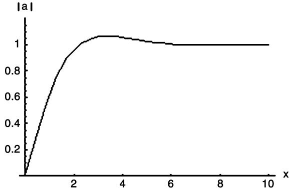
Fig. 8.7 A plot of the function |a(x_3)| against x_3 . This plot has a peak of 1.06702 at x_3 = 3.33216 and then it is asymptotic to the value one as x_3 tends to infinity
