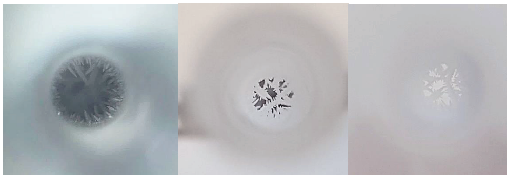
Figure II-13. Pictures of \text{NH}_4\text{NO}_3 ammonium nitrate solidified on inner tube walls during Fast SCR conditions.
