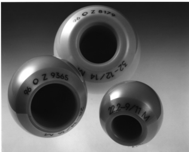
Figure 10.30 Laser markings of zirconia femoral ball heads (Heimann and Willmann, 1998). For details, see the text.
