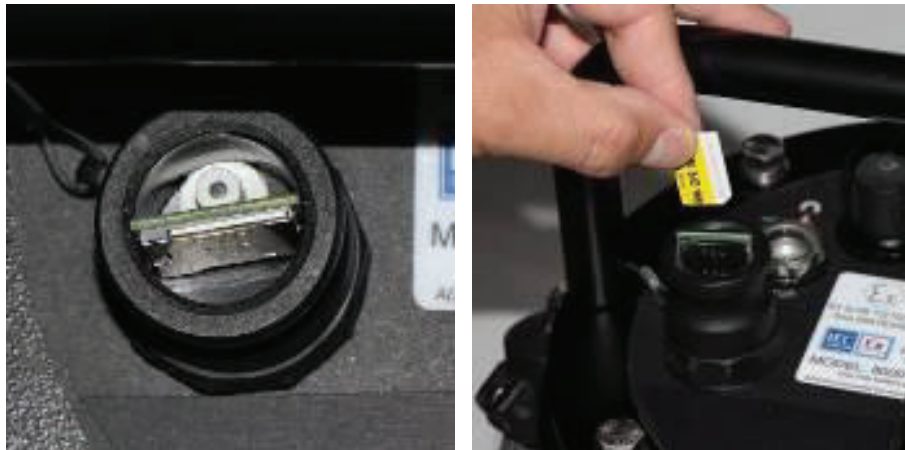
Empty SIM card holder showing pressure valve (left); inserting the SIM card properly into the holder
