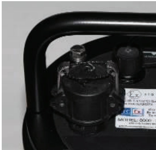
SIM card enclosure with plastic tie
