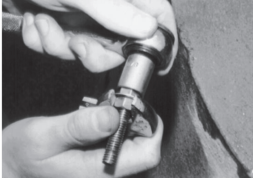
Binding the nuts together with the washer in between
