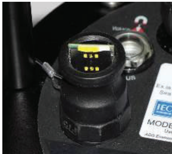
SIM card properly seated and secured in the holder
