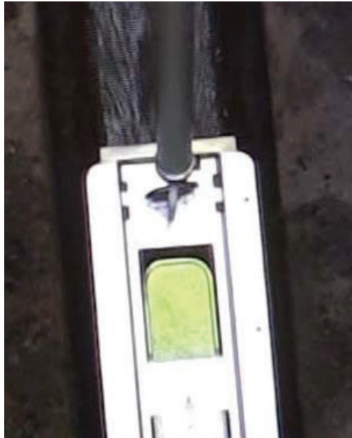
Position the Hook Through the Loop on the Sensor Bracket
