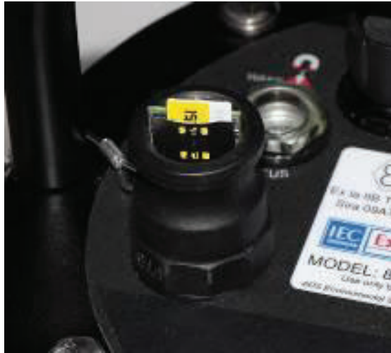
SIM card slightly ejected from its secure position in holder
