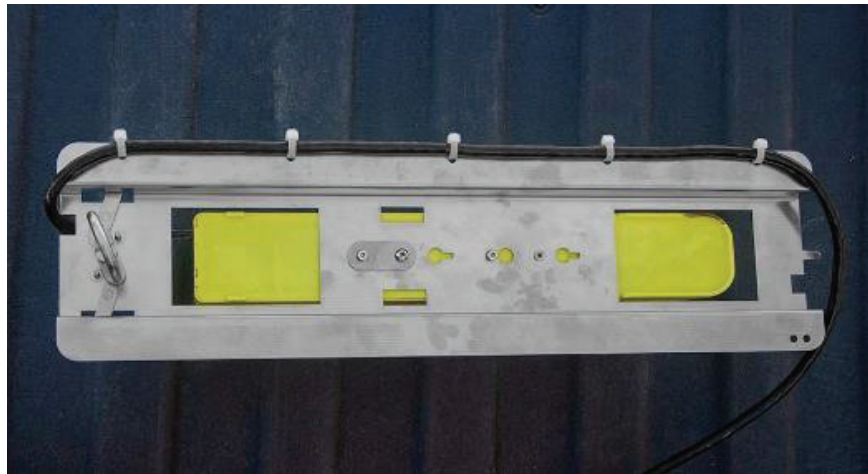
Cable Tie Sensor Cable to Sensor Bracket
