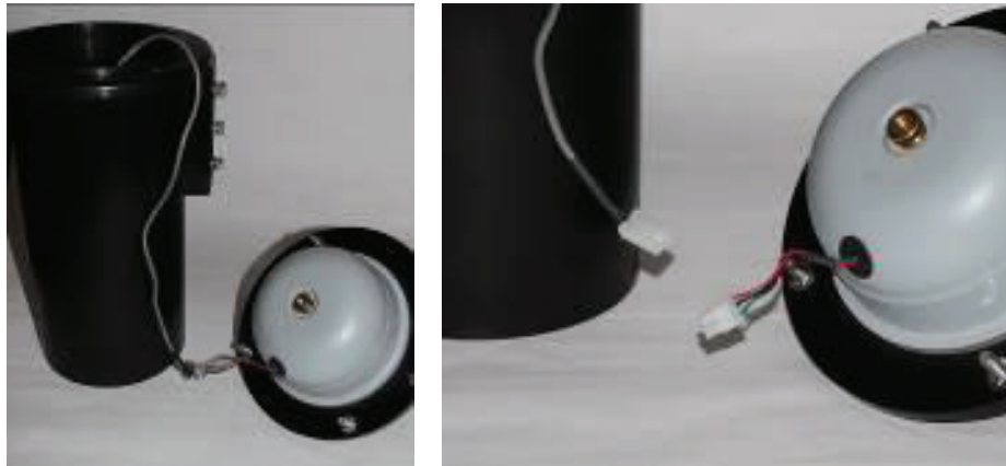
Placing the top next to the monitor (left) and disconnecting the cables at the plastic white connectors (right)
