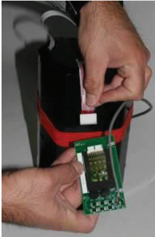
Disconnecting the PCB from the battery pack
