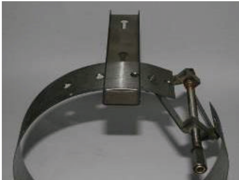
Properly attached spreader mechanism (with Ultrasonic Depth Sensor mounting plate on ring)
