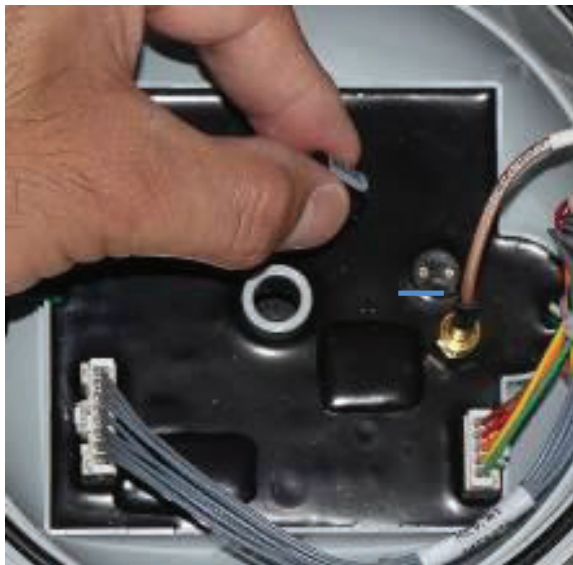
Blue fuse removed from the regulator board
