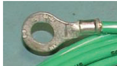
Ground wire ring terminal from ground cable
