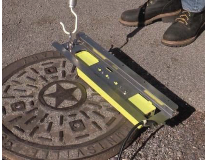
Sensor Bracket Securely Looped on Pole Hook
