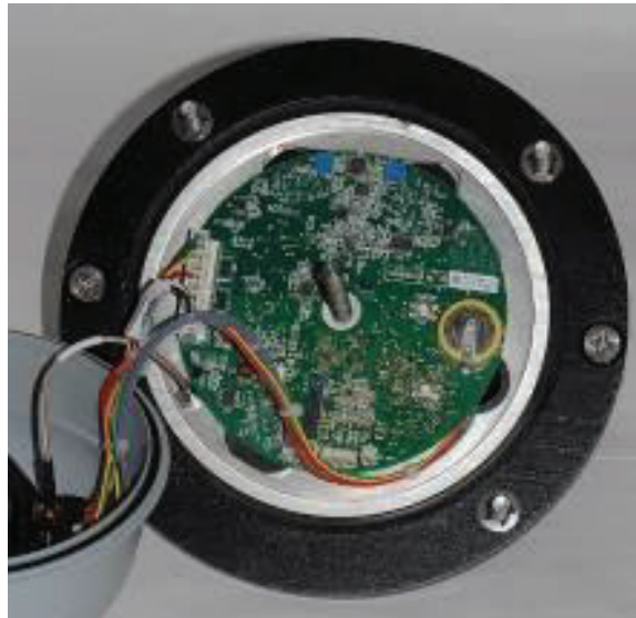
TRITON+ top with processor board attached
