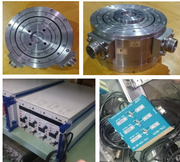
Figure 10: Izumi multicomponent load cell and apparatus
