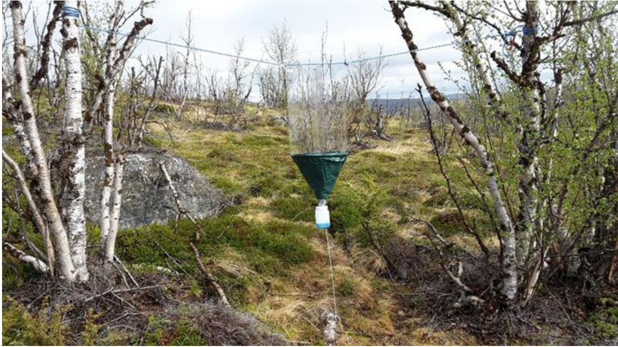
Figure 3: One of the window traps used in this study shortly after it was assembled (Photo: Petter Carlsen).
