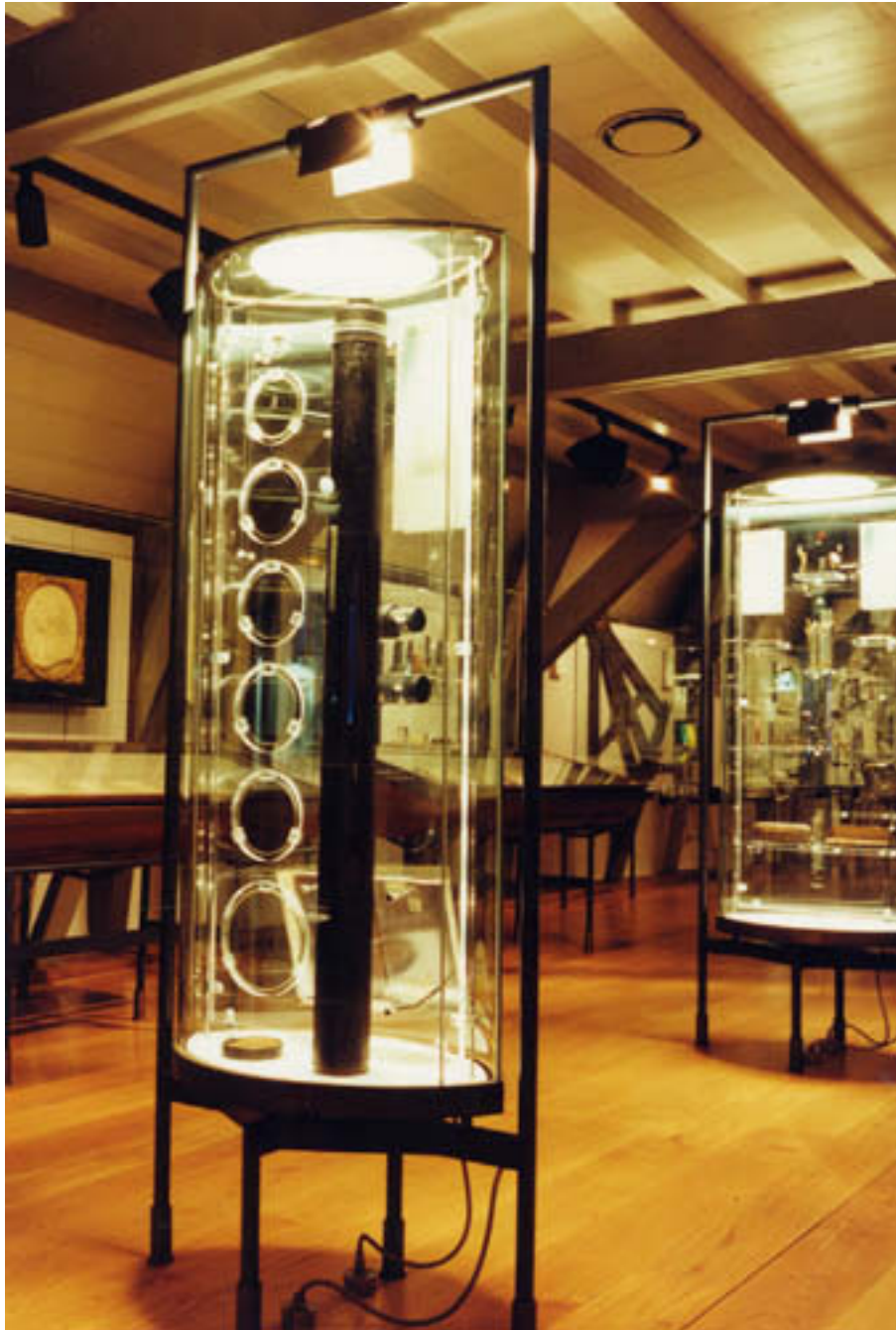
Figure 16: The 'Campanine' telescope displayed standing vertically. The 5 metal drawtubes of the telescope are pushed in.
