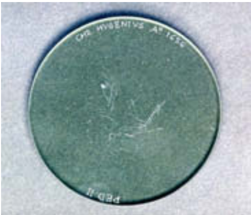
Figure 5: Here we see an objective lens made by Christiaan, similar to the one he used to discover Saturn's moon 'Titan'. Along the rim Christiaan signed: "Chr. Hugenius A° 1656". On the opposite side of the lens "PED II" tells us the focal length is 11 feet. (Lens from the Louwman Collection of Historic Telescopes; photo by author; also Figure 6)
