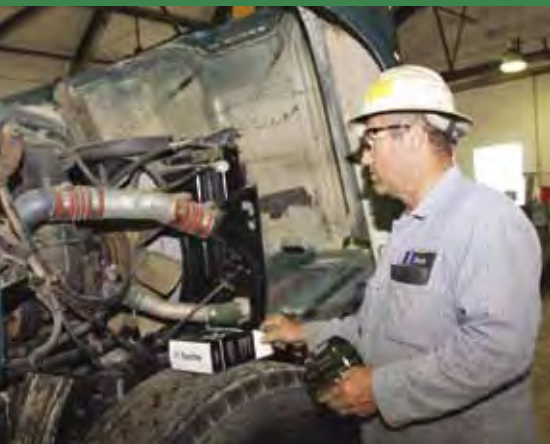
Tim Lemasney performs a Department of Transportation (DOT) inspection on a fuel truck, fixing the exhaust pipe so it's ready to be sent out to jobs.
