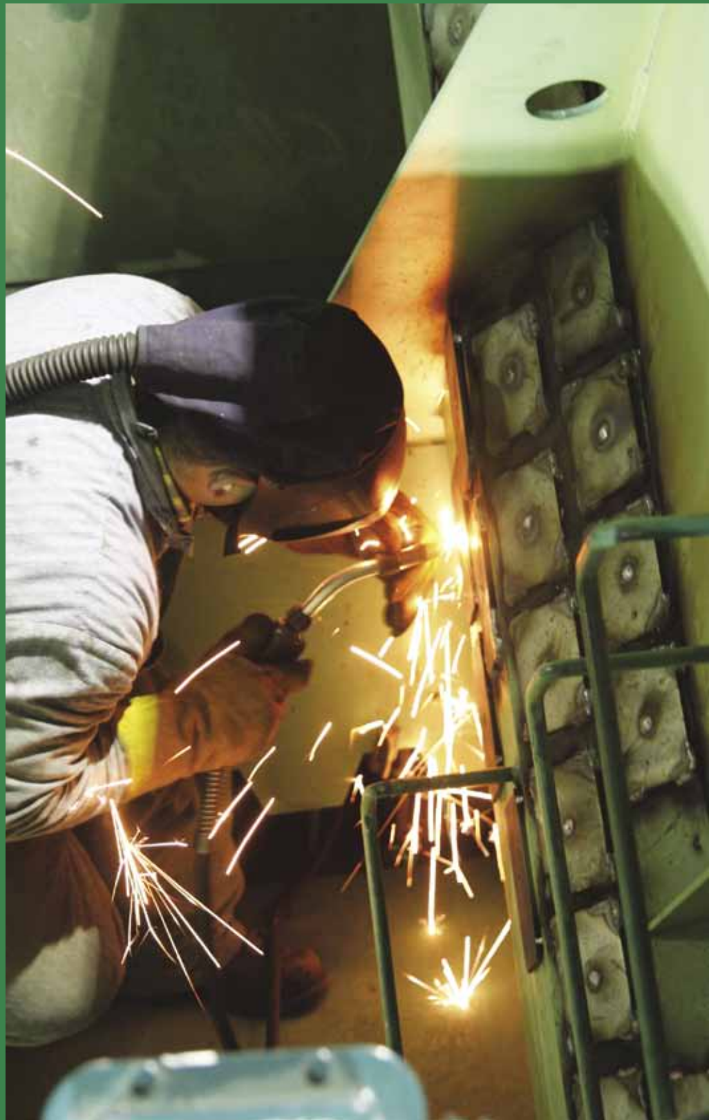
Third-step Apprentice Tyler Rose welds a wear plate into a shuttle buggy. "I've done a lot here – just whatever they need," he said, explaining that he got into the field because he likes being outside.
