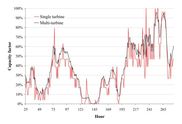
Figure 63: Capacity factors for a single turbine and a multi-turbine approach, estimated from wind-speed data
