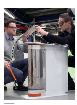
Slat with Electric Ice Protection Systemdemonstrator tested in icing tunnel to demonstrate TRL4 maturity level.
