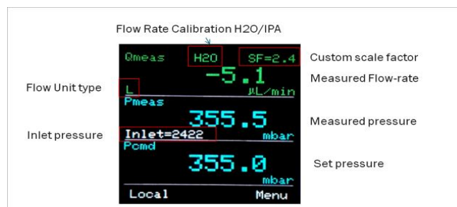
Figure 4: Control window of the Flow EZ™.
