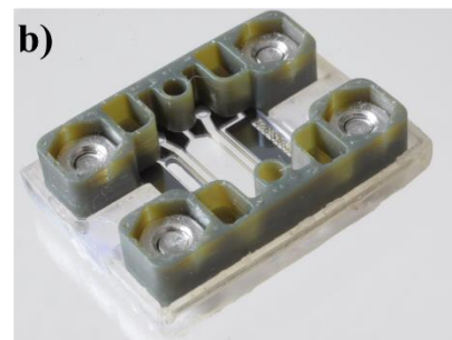
Figure 2: A typical assembly of a microfluidic chip and holder ( \sim 3 \times 2 \text{ cm}^2 ). The chip is sandwiched between two 3D-printed parts, which are fixed by M3 screws. Liquid reservoirs, connected with O-rings to the chip, are integrated in the top holder. a) A schematic, and b) a photo of the device.
