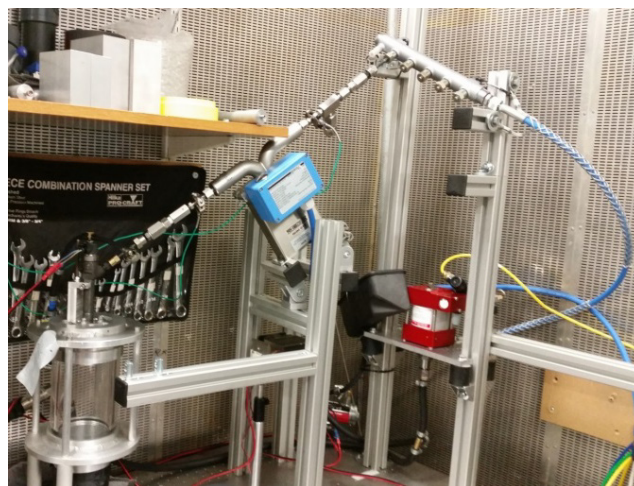
Figure 3: Experimental set up: high pressure diesel fuel line, Coriolis flowtube, injector, cylinder.
