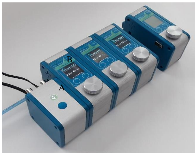
Figure 8: LineUP™ system. A: Link module. B: Flow EZ™ module.
