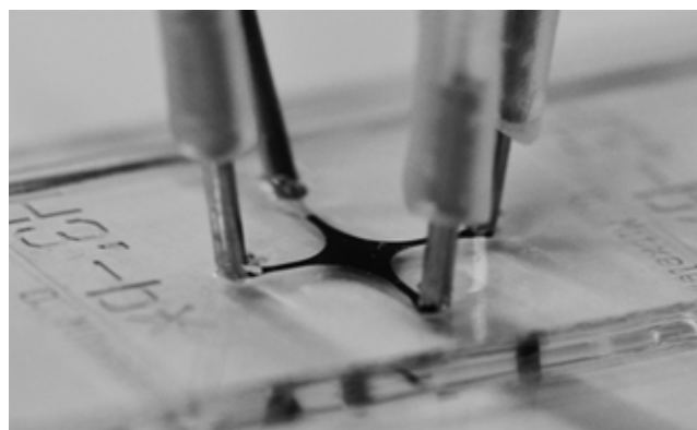
Figure 1: Real PDMS-glass microfluidic platform filled with ink and with the corresponding connectors [14].
