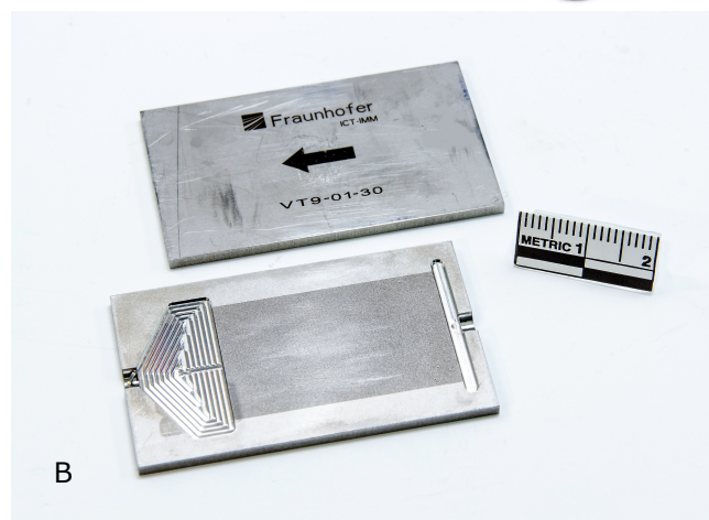
Figure 1: Example of a microchannel evaporator used for vapor generation in laboratory-scale applications. A): complete complete evaporator an B): internal structure.
