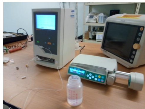
Figure 1: Infusion pump analyzer (on the left) and a syringe pump (on the right) during a calibration
